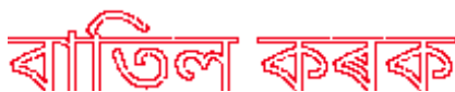
Figure 4: Pixel delta (marked in red) for a bootloader image containing a multilingual info message.
